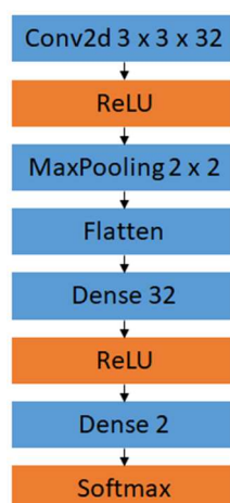
Figure 2: Architecture for the simulation study
